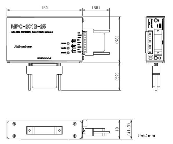
\*This unit can mount on the metal surface with the magnet.
