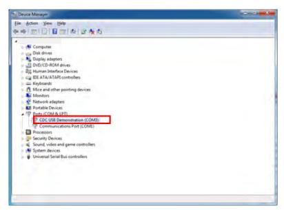
2-10. Check the assigned port number because the CDC USB Demonstration (COMxx) is used for communication setting. Note: Assignment of COM port depends on the PC to use.
