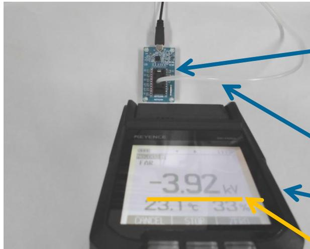
When the ionizer is **used**: **-1V**
