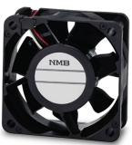
NMB Technologies provides Ingress Protection (IP) rated cooling fans – IP55 provides dust proof and protection against harsh environments and is for outdoor applications. These 60mm to 120mm IP55 rated fans are available in 12V, and 24V with tacho output for speed monitoring. Fans are outfitted with NMB precision machined stainless ball bearings for long life, corrosion resistance and high reliability.
