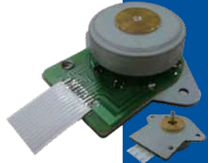
■ 3 Phase outer rotor type DC Brushless Motor
