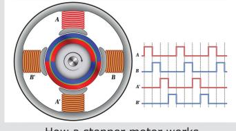
How a stepper motor works
