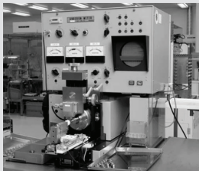
Anderon Meters are used to test vibration noise. All ball bearings manufactured by MinebeaMitsumi undergo vibration testing.
