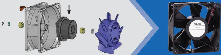
In addition to protection from external contaminants, NMB's IP69K fan are available with pulse-width modulation (PWM) speed control. Our customers can expect longer fan life with PWM speed control - the fan will spin faster only when required, thus reducing bearing load and wear. Power consumption will also be reduced because the fan will demand less power draw according to the duty cycle required.
